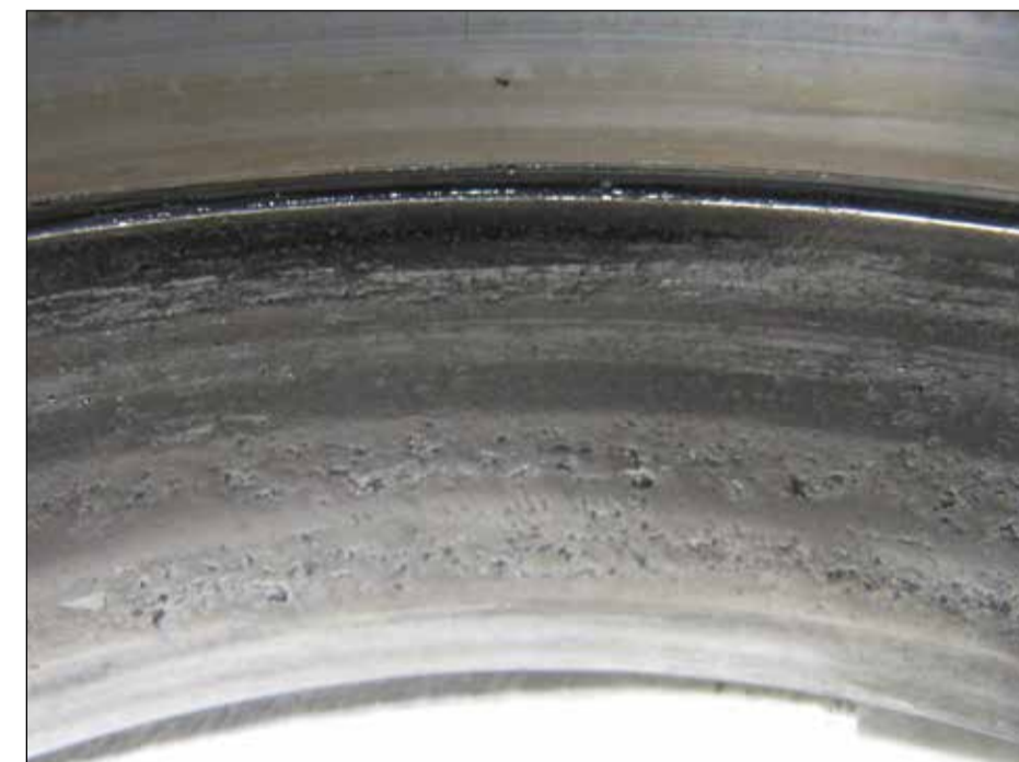
Premature wheel bearing failure
